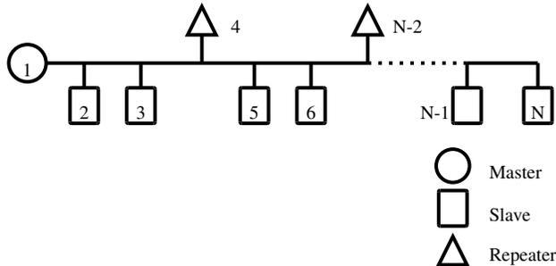
Fig. 1. Topology of network with repeaters
