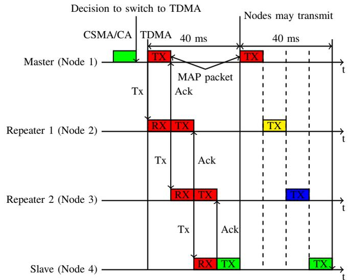
Fig. 2. Switching process from CSMA/CA to TDMA with repeaters
