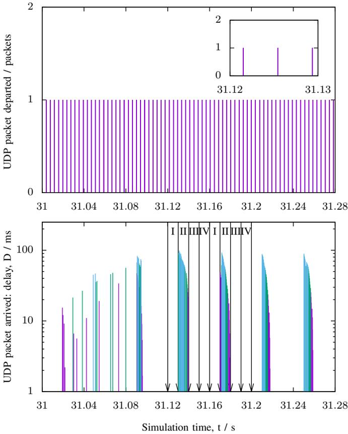
Fig. 3. Uplink delay for UDP packets with ALS and 2 repeaters,  $N=4$ , G.hn
