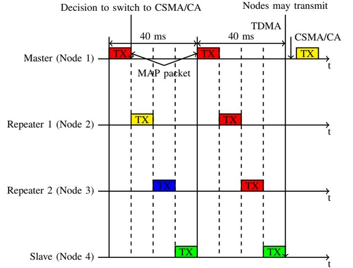
Fig. 4. Switching process from TDMA to CSMA/CA with repeaters
