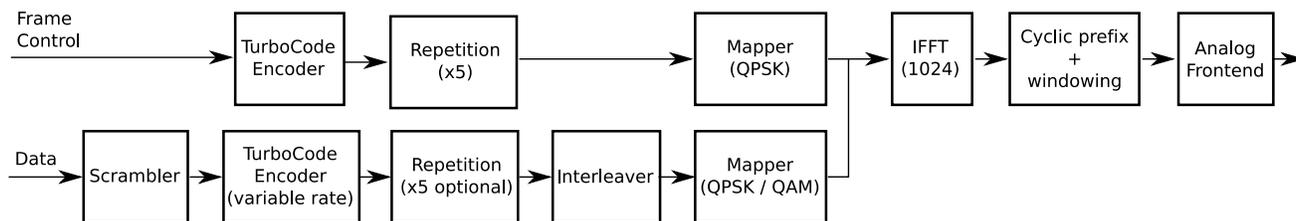
Figure 1. PHY layer transmission structure
