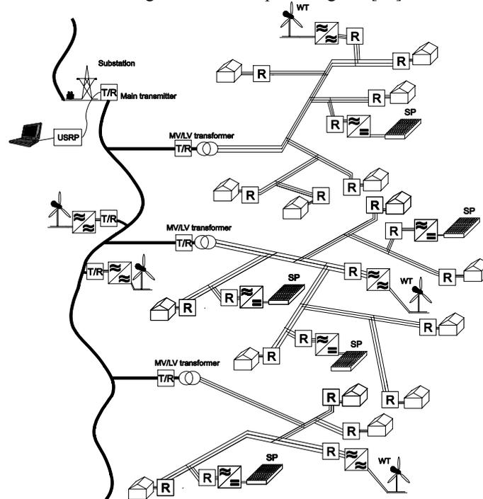
Fig. 1 Typical distribution network from the electrical substation to the customers with DGs; solar panels (SP) and small-scale wind turbines (WT), and the proposed anti-islanding protection system with a transmitter (T) and receivers (R) in an MV-LV grid.
