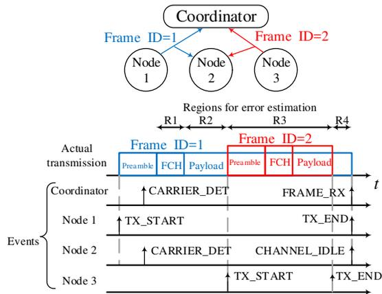
Fig. 1. Simplified transmission example and corresponding events and regions used for errors estimation.
