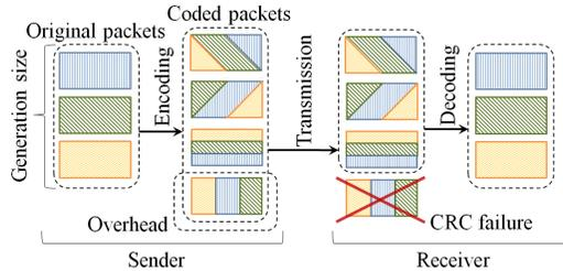
Fig. 1: Data transmission with NC [3]
